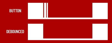
Debouncing an input refers to filtering out very short presses sometimes with a capacitor or in this case with some code.
